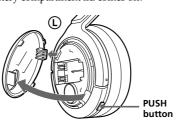
2 Insert the supplied rechargeable nickelmetal hydride battery into the battery compartment matching the  $\oplus$  terminal on the battery to the  $\oplus$  mark in the
